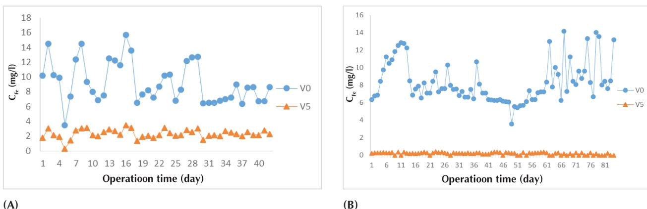
**Fig. 4. Removal of iron in the second and third operated mode.** (A) The second operated mode; (B) the third operated mode. Note: V0 - groundwater; V5 - treated water.
